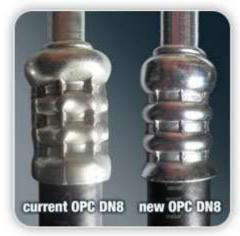
Thanks to the more compact dimensions, the more limited deformation of the ferrule during the crimping determines a more homogeneous folding of the steel giving a better and regular compression of the rubber wall of the hose.
